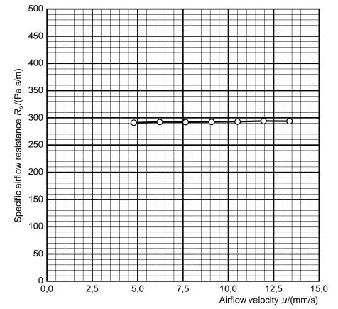
Specific airflow resistance  $R_s(0.5 \text{ mm/s}) = 290 \text{ Pa s/m}$
