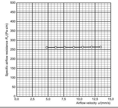
Specific airflow resistance  $R_s(0.5 \text{ mm/s}) = 260 \text{ Pa s/m}$
