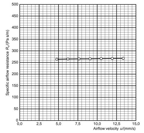
Specific airflow resistance  $R_s(0.5 \text{ mm/s}) = 262 \text{ Pa s/m}$
